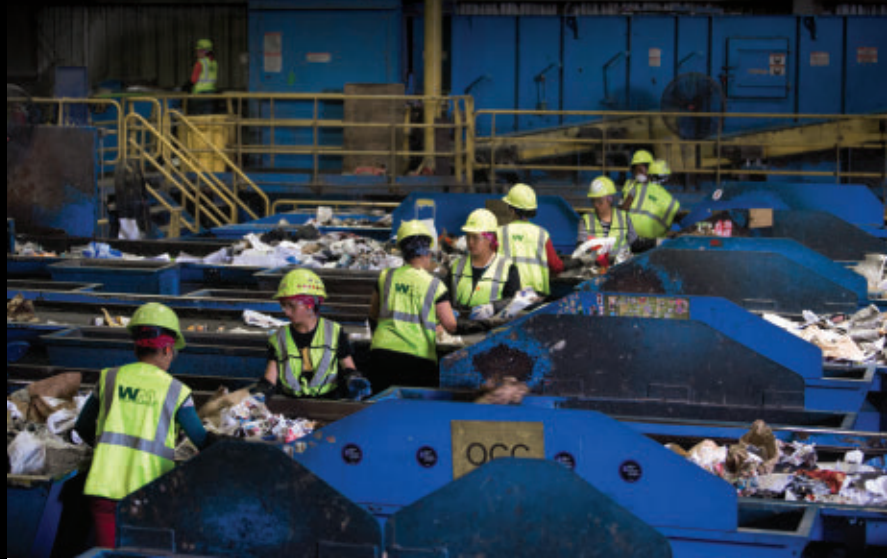
At the Waste Management Material Recovery Facility in Elkridge, Md., workers sort trash moving past them on conveyor belts.
