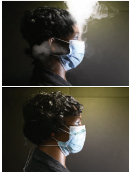
Aerosols can spew from gaps where medical masks don't fit the face (top, as demonstrated on a manikin). A mask fitter worn over such a mask can prevent that leakage (bottom).
