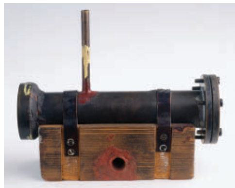
Physicist James Chadwick used this device to discover the neutron in 1932, based on radiation emitted after beryllium was hit with alpha particles, the nuclei of helium atoms.
