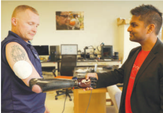
Retired U.S. Army Sgt. Garrett Anderson shakes hands with researcher Aadeel Akhtar, CEO of Psyonic, a prosthesis developer (left). A wireless skin patch on Anderson's upper arm gives him sensory feedback when grasping an object. Inside the patch are circular actuators that vibrate in response to signals. The prototype device (right) might give the sensation of touch pressure in artificial limbs, in virtual reality and telemedicine.
