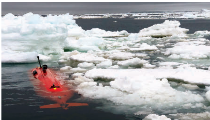
Ocean data collected by this red autonomous underwater vehicle from beneath the Thwaites ice shelf in Antarctica are helping scientists identify sources of warm water eroding the ice.
