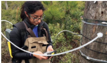
Ecologist Melinda Martinez uses a portable gas analyzer to measure “tree farts” in a ghost forest.
