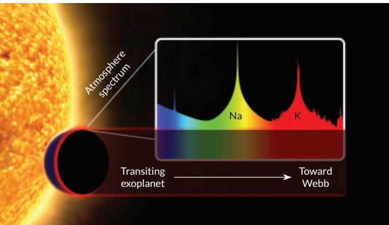
**Transit advantages** Webb will measure the composition of exoplanet atmospheres by looking at the light from the planet's host star as the planet crosses in front of the star. Atoms and molecules in the atmosphere, such as sodium (Na) and potassium (K), absorb certain wavelengths of the starlight, leaving a unique fingerprint in the spectrum of light that reaches Webb's detectors.
