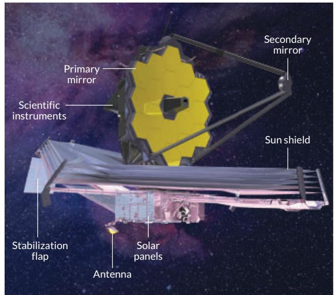
**A novel design** Once all is unfolded, the James Webb Space Telescope’s sun shield will span the length of a tennis court to protect the main and secondary mirrors from the sun, moon and Earth’s light and heat. The solar panels, exposed to the sun, will convert light to electricity to power the instruments. Webb’s antenna will keep it communicating with scientists on Earth, sending data from the scientific instruments. The stabilization flap keeps the machine from veering off course.
