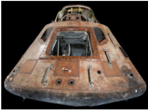
Astronauts in the Apollo 11 command module (left) were protected from high temperatures during re-entry through Earth’s atmosphere (center) by a heat shield made of Avcoat, a reinforced plastic made from an epoxy resin within a honeycomb fiberglass network. A new NASA spaceship called Orion, destined to take people to the moon and beyond, uses Avcoat tile blocks bonded onto its heat shield (right).
