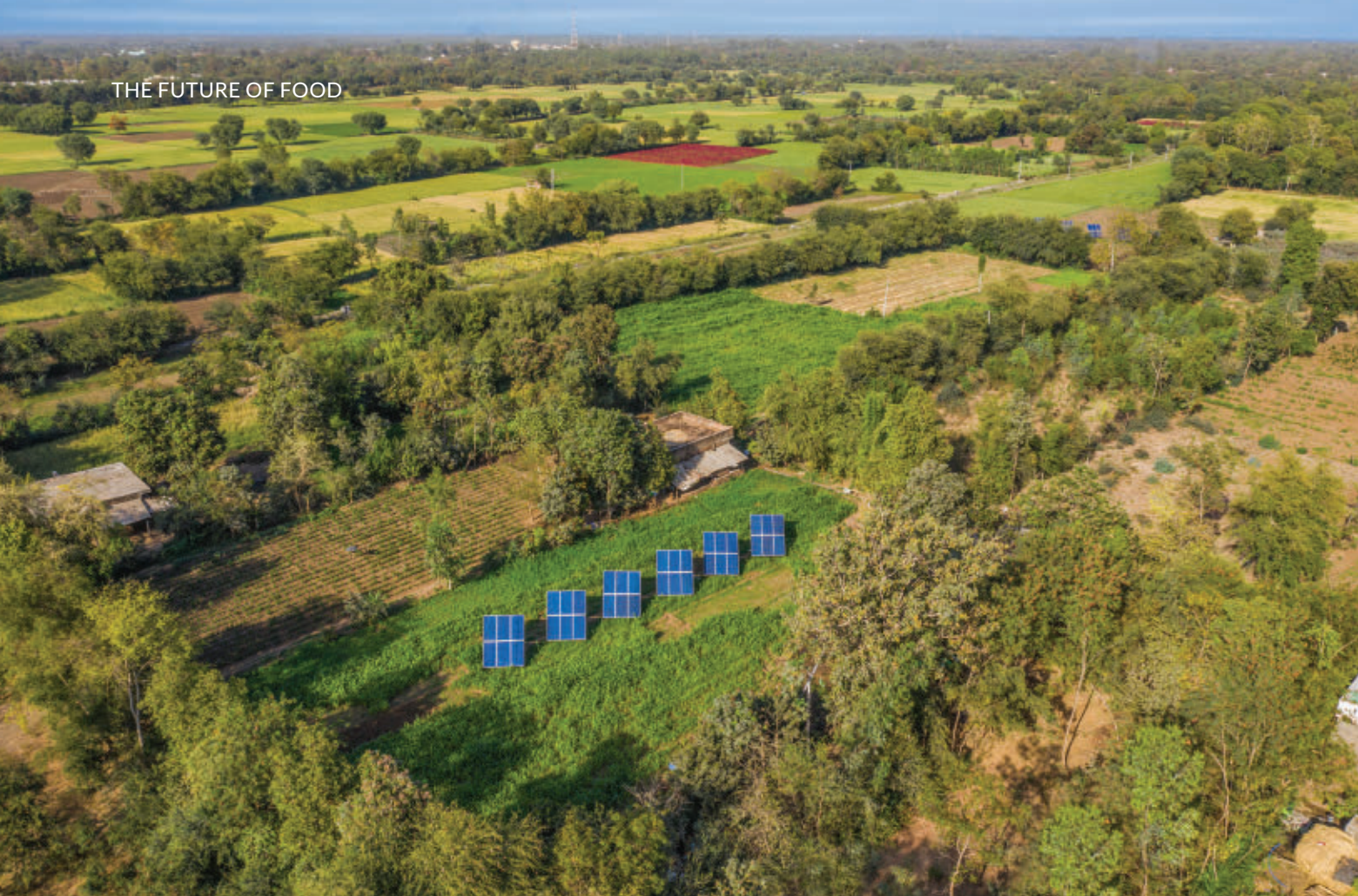
This aerial image shows solar panels installed among crops to power groundwater pumps and offer a new income source for farmers in western India's Dhundi village.
