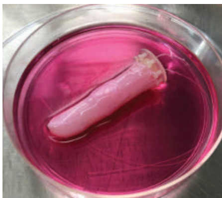
This robotic finger spent much of its time in a nutrient bath to keep its skin suit healthy.
