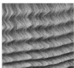
RESILIENT RIPPLES An electron micrograph shows how aligned carbon nanotubes buckle at their bases after 1,000 compression cycles. Above this region (not shown) the tubes remain straight.
