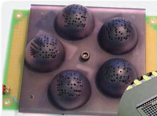
BUG EYES — Peering through pierced domes, a prototype motion tracker generates coordinates instead of an image. Inset: A lenslet array marries unconventional optics and digital processing to make a detailed image despite the device's microchip size.
