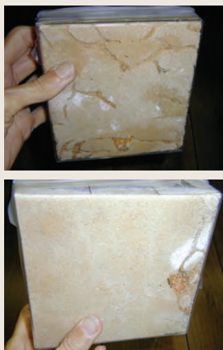
LINE IN THE SAND Termites burrow readily through untreated sand (top) but not through sand treated with catnip oil (bottom).
