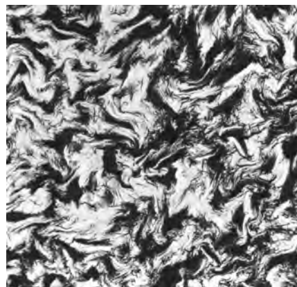
ALLOY THERE A new titanium-based alloy containing four other elements has a marbled microstructure after the material is deformed through compression.
