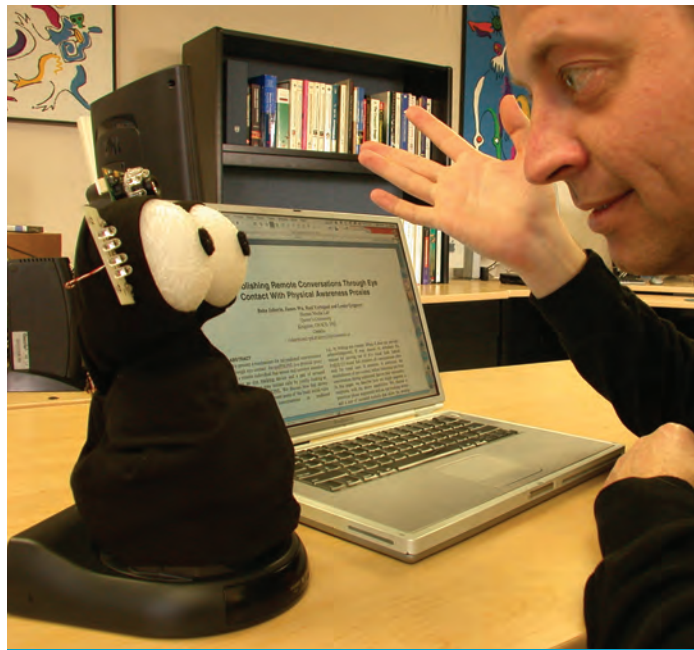
STARE MASTER — An eyePROXY telephone controller seeks eye contact as the go-ahead to put through an incoming call.
