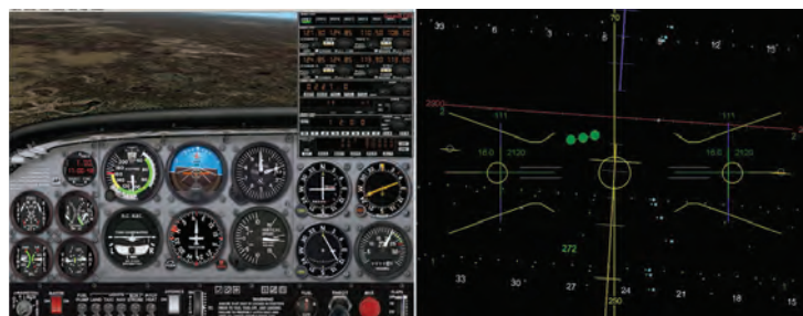
IN PLANE VIEW — A typical cockpit setup, left, contrasts with that of the OZ system, right. OZ combines data from dials and gauges into a visual depiction of the aircraft and external conditions. Here, the aircraft approaches a runway, represented by three green dots.
