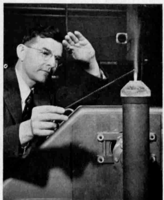
ELECTRONIC TORCH —Dr. J. D. Cobine of the General Electric Research Laboratory melts a quartz rod in the flame of an electronic torch so hot that it will melt firebrick and tungsten, the latter of which melts at 3370 degrees Centigrade. The flame consists of nitrogen being passed through a high-frequency arc.
