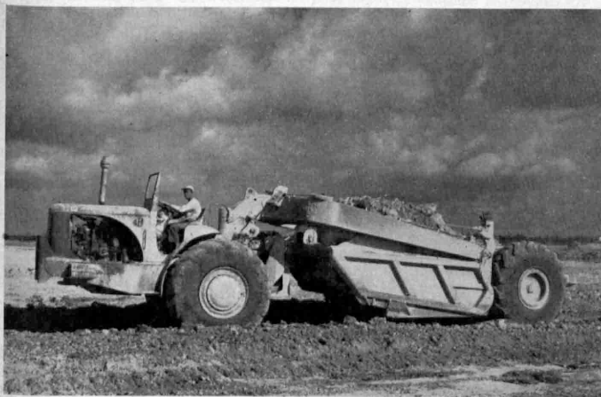
TURBOCHARGED DIESEL —Picking up a heaped load of 18 cubic yards of earth at high speed is a specialty of this International Harvester pay scraper. It is powered by a 262-horsepower turbodiesel built by Cummins Engine Company, Inc. Turbocharging harnesses exhaust gases normally wasted.
