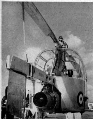
ULTRA-LIGHT HELICOPTER —This plane is powered by compressed air supplied to pressure-jet units at tips of two-bladed rotor. Pilot and observer sit facing forward or aft with a 360 degrees field of vision. The helicopter can be transported on a three-ton truck.
