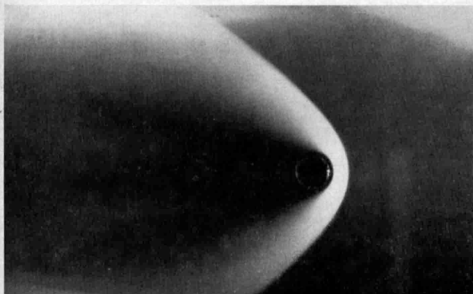
HIGH ALTITUDE FLOW —Picture of low pressure air rushing over a cylinder in the University of California's high altitude wind tunnel indicates that supersonic planes may encounter greater heat problems above 20 miles than they do near the ground. The reason is that air is more viscous at such high altitudes. (See SNL Oct. 15, p. 248.)
