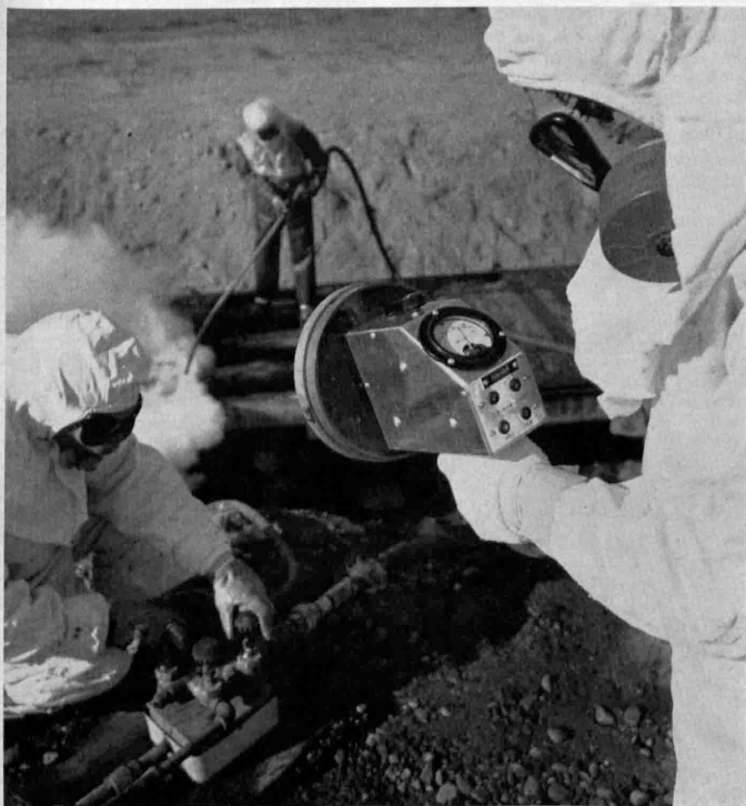
ATOMIC RAY DETECTORS —Overcoming disadvantages of conventional detectors, this new wide-angle atomic ray detector developed by General Electric scientists is used to monitor radioactive material being removed from flatbed trucks with caustic steam.
