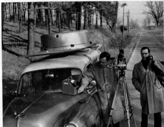
SAMPLING FOR HIGHWAY VISION —To measure the light scattering and absorption characteristics of fog, research engineer Benjamin Pritchard, on the left, and Dr. H. R. Blackwell, director of the University of Michigan's vision research laboratories, use the equipment shown here. Domed device atop the instrument-crammed station wagon makes possible mile-by-mile record of the way fog reflects light. The studies are aimed at improving highway vision.
