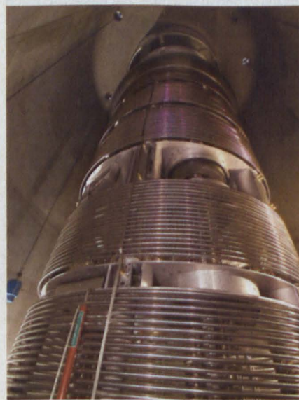
HOT HOOPS High-voltage tubes shown encircling this electron accelerator drive cooling electrons downward to join with antiprotons in the world's highest-energy particle collider.
