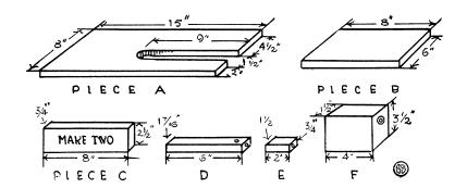
into the end 2 inches deep, and a 5%-inch hole through it the thin way, an inch from the end, and intersecting the 5/16-inch hole. In the large board, piece A, cut a slot 1½ inches wide and 9 inches long, 2 inches from one edge. All these pieces are illustrated. They may be made of most any kind of wood.
