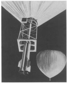
ROCKET VEHICLE—At the launch altitude for the Far Side rocket vehicle, developed by Aeronutronic Systems, Inc., Los Angeles, the 3,750,000-cubic-foot balloon is fully inflated to its maximum diameter of 200 feet. The full view of the complete assembly shown at the lower right gives an idea of its comparative size. The balloon launching is being made in an effort to free rockets from the high friction of lower atmosphere and to preserve their power for outer space.
