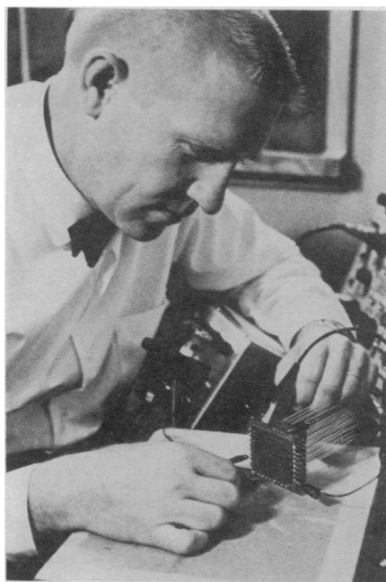
INFORMATION STORE —A network of magnetic "pins" the size of a cigarette package, tested here by D. A. Meier, is said to be able to store 8,000 "bits" of information.
