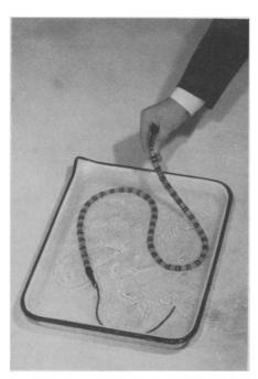
ELECTRIC "EEL"—A snake-like assembly of tiny battery cells that can be wound on a drum along with the cable, is activated when unreeled into water. Rubber rings separate silver chloride links from zinc segments. Developed for the U.S. Army Signal Corps by Aerojet-General Corporation, Azusa, Calif., the snake batteries are spliced into cable every mile to boost voice or teletypewriter signals.
