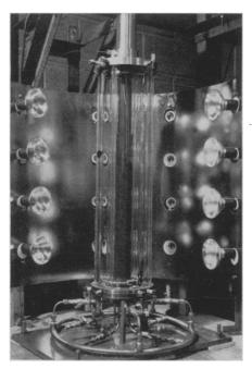
GROWING ALGAE—Glass cylinder for growing algae is cooled by refrigerated ferrous sulfate solution circulated through a space outside the algae chamber to reduce heat from lamps.
