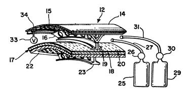
One past technique has been to use fuel tanks with an inner and outer wall, with the space between the walls filled with a noncondensable gas, usually helium. Unfortunately, the helium raises the thermal conductivity of the insulation, which necessitates a greater weight of insulation to keep the hydrogen in its liquid state.
