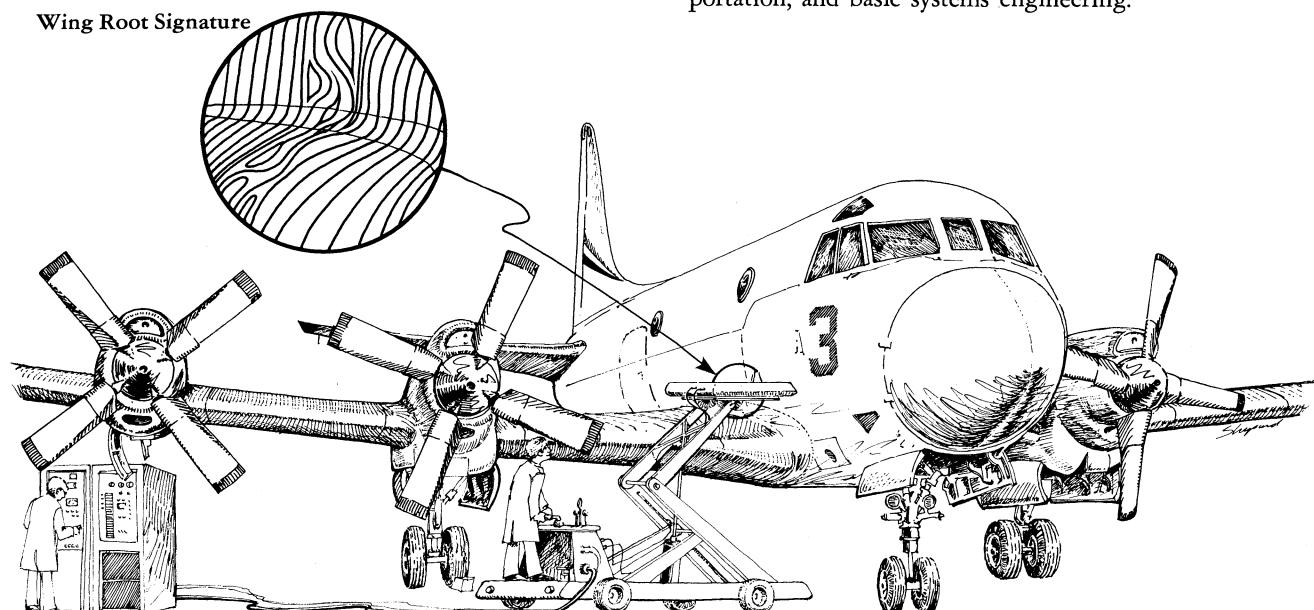
The first tests were conducted in a TRW lab, however, where wing panels from a P-3 patrol plane were inspected. The prototype holographic systems not only found every flaw that had been previously located by conventional methods but also found several that had not been detected at all.
