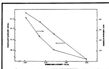
NO<sub>x</sub> emissions have long been a major concern in the operation of hydrogen-fueled engines. Now, however, Swain and co-workers have detailed a computer analysis of a theoretical hydrogen engine that can reduce NO<sub>x</sub> emissions. In the computer study, the researchers determined the extent to which a hydrogen-powered engine — modeled after a Pontiac Sunbird — can be “leaned out.”
