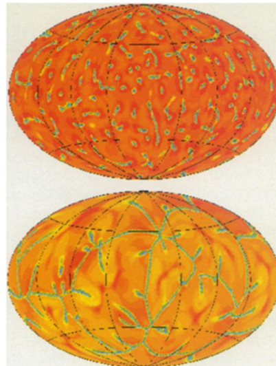
In a model of Earth's mantle, reds show rising rock and greens denote sinking material. When the viscosity of the mantle is uniform from top to bottom (top), the model produces a blotchy convection pattern. Increasing the lower mantle's viscosity leads to larger, more realistic convection cells (bottom).
