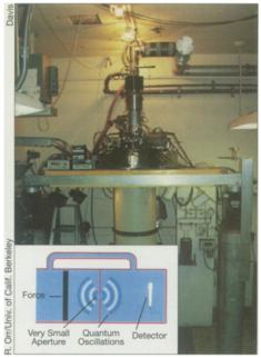
Special refrigerator used to chill helium-3 to less than 1 millikelvin. Inset: In this drawing of the apparatus, a force causes a slight pressure difference between two reservoirs of the superfluid, which induces it to oscillate through a tiny aperture, generating waves that can be picked up by an extremely sensitive detector.
