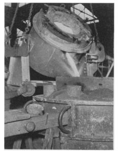
wall heats the 1000-pound charge. The outfit does away with superheating the metal and eliminates preheating the transfer ladles.
