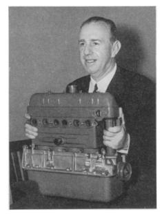
COMPACT ENGINE—The new 26-horsepower Crosley engine is built on a radically new principle from thin sheet-steel stampings and weighs only 59 pounds. Holding the engine easily on his lap is Powel Crosley, Jr., president of Crosley Motors, Inc.
