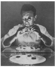
AUTOMATION AIDE—Skilled human fingers wire small, circular core units that serve as "nerve" cells for a new switch expected to stimulate assembly-line automation. Nicknamed "magnetic detective" by its developers, electronic engineers at Minneapolis - Honeywell's Doelcam Division, the new switch can monitor an assembly-line sequence of parts containing metal to confirm each piece and move it on, or shut down the assembly line if needed.
