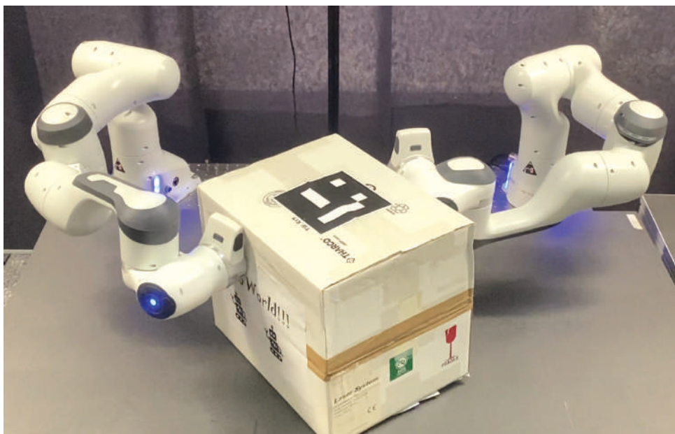
Robots can benefit from tensor networks too. Scientists used tensor networks to enable these two robotic arms to rotate and lift a box. Structuring data in tensor networks can allow for more efficient robot training than standard methods.
