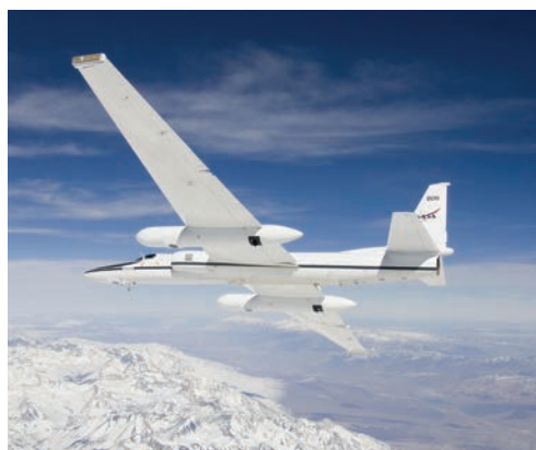
NASA uses the ER-2 research aircraft (bottom right) to conduct experiments at altitudes up to 21 kilometers, such as this flight above California (top). Pilots must wear pressure suits (bottom left) because a loss of cabin pressure could cause them to lose consciousness within seconds and quickly die.
